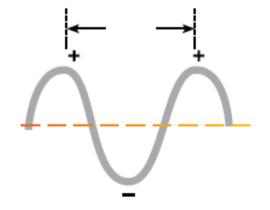
Radio waves oscillate, or flip back and forth, between plus and minus at a predictable rate.
