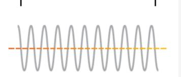
The number of cycles in one second gives the frequency. How "frequently" the signal oscillates in one second.
